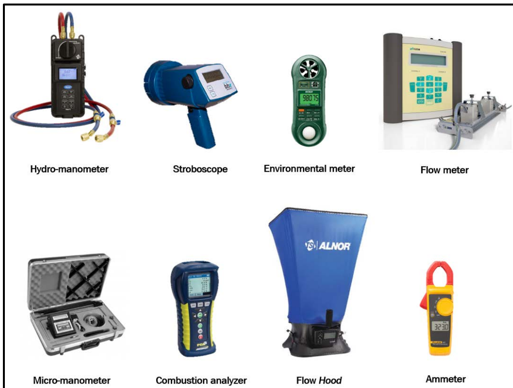
Figure 30. Typical RCx functional test tools.
